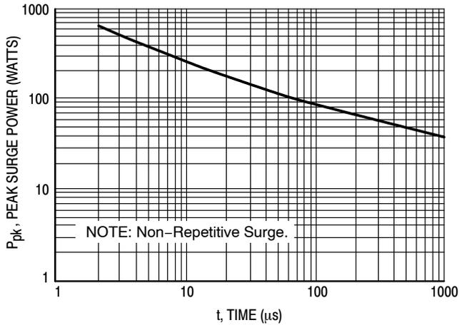
Figure 1. Peak Power Dissipation versus Pulse Width
