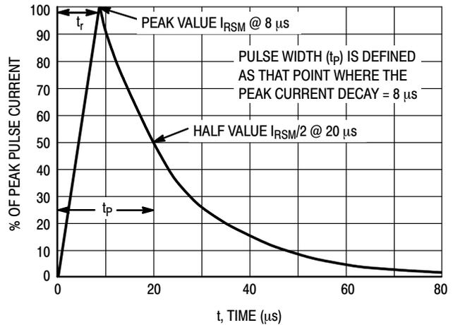
Figure 2. Pulse Waveform  $8 \times 20 \mu\text{s}$
