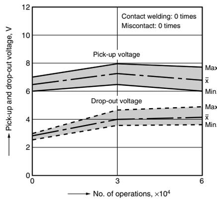
**2-(3). Inrush 70.7A, Steady 20A, 250V AC electrical life test (Compressor dummy load)**
