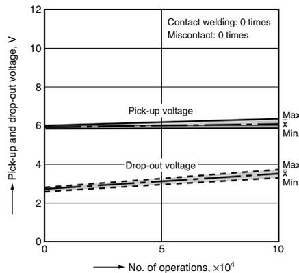
**2-(4). Electrical life test (20A 250V AC, resistive load)**
