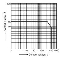
2. Max. switching power (DC resistive load)
