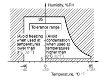
4) Condensation Condensation forms when there is a sudden change in temperature under high temperature and high humidity conditions. Condensation will cause deterioration of the relay insulation.
