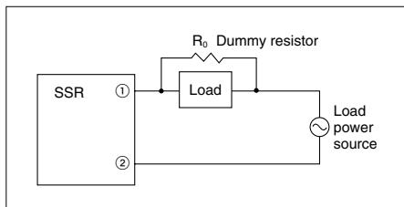
In case the dummy resistor is not used, keep in mind that the residual voltage becomes as follows:
