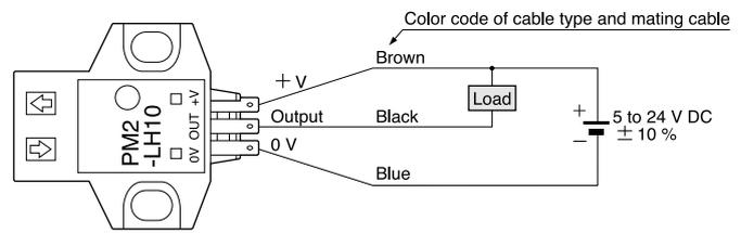
Note: Make sure to connect terminals correctly as the sensor does not incorporate a reverse polarity protection circuit.
