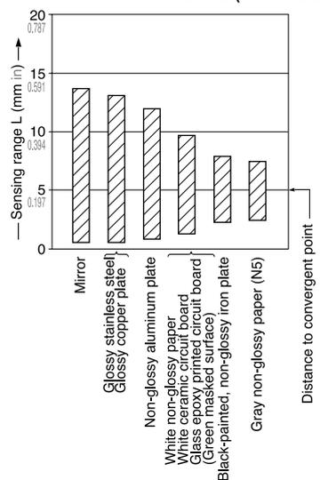
The bars in the graph indicate the sensing range for the respective material. However, there is a slight variation in the sensing range depending on the product. Further, if there is a reflective object (conveyor, etc.) in the background of the sensing object, since it affects the sensing, separate it by more than twice the sensing range shown in the left graph.
