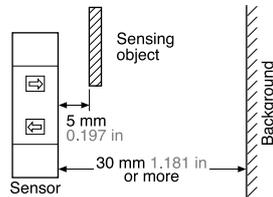
(However, the specular background should be a plane surface, directly facing the sensor. A spherical or curved background may be detected.)
