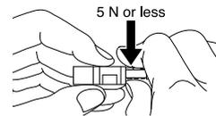
Caution: Be sure to hold a connector when plugging or unplugging it. Do not hold a terminal or a cable when plugging or unplugging the connector. Otherwise, it will cause a poor contact.
