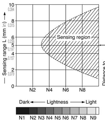
The sensing region is represented by oblique lines in the left figure. However, the sensitivity should be set with enough margin because of slight variation in products.
