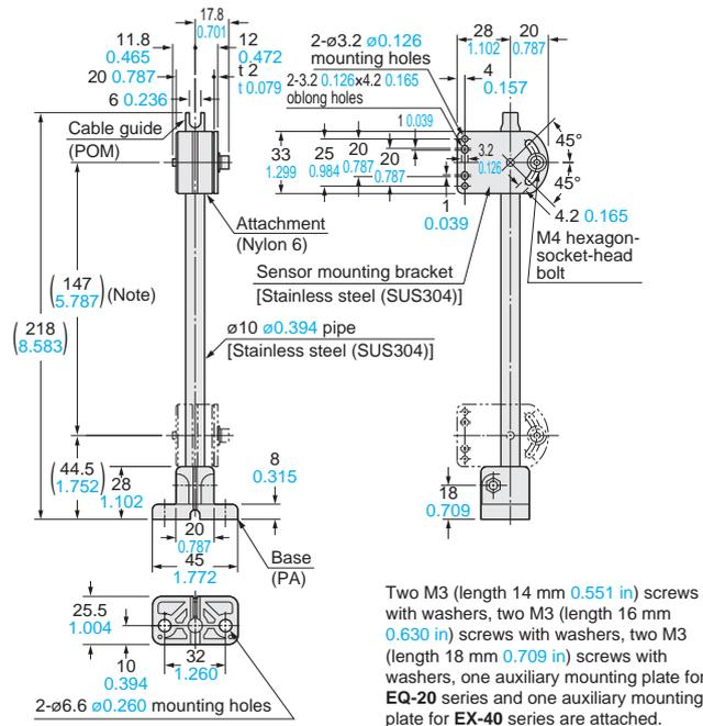
Note: The dimensions in the brackets indicate the adjustable range of the movable part.
