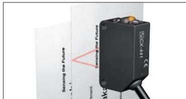
Thanks to its unique optics and specialized design, the **CX-400's** electronic circuits allows for consistent sensing of minute 0.4 mm **0.016 in** (the thickness of a business card) differences or 10  $\mu$ m **0.394 mil** ultra-thin film.
