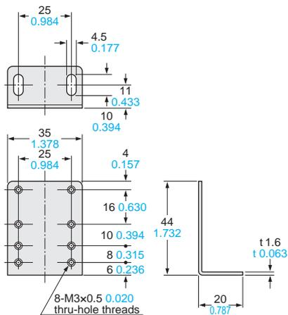
Material: Cold rolled carbon steel (SPCC) (Uni-chrome plated)
