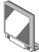
Two M4 (length 10 mm **0.394 in**) screws with washers are attached.
