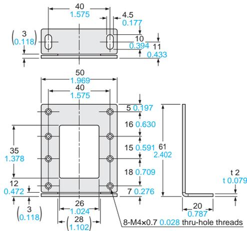
Material: Cold rolled carbon steel (SPCC)
