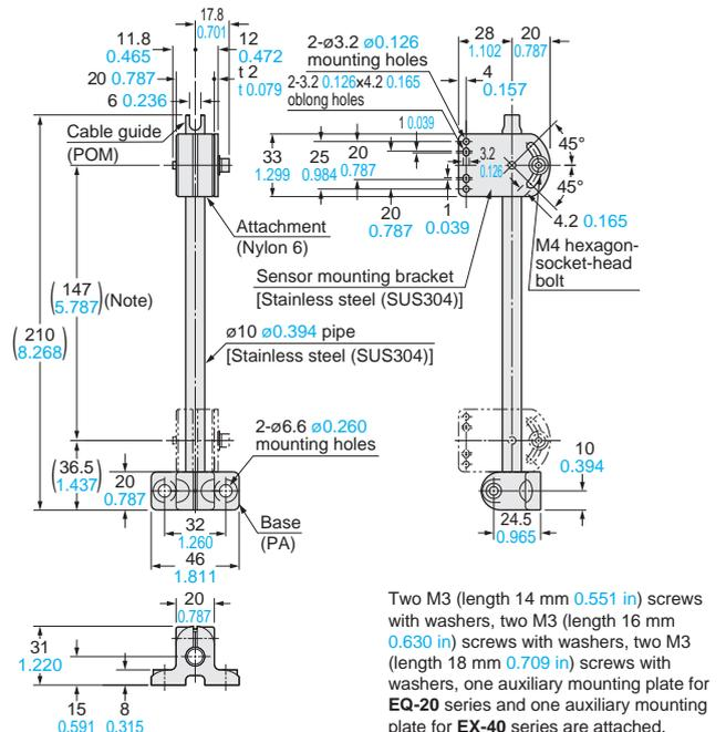
Note: The dimensions in the brackets indicate the adjustable range of the movable part.
