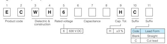
Rated voltage 630 V.DC (Odd size taping)
