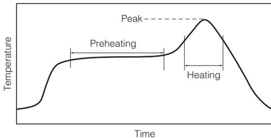
For soldering (Example : Sn/Pb)
