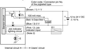
Symbols ... D : Reserve supply polarity protection diode Z<sub>D</sub>: Surge absorption zener diode Tr: PNP output transistor
