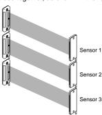
· However, if the sensors are mounted close together as shown in the figure below, up to 2 sets of sensors are possible.
