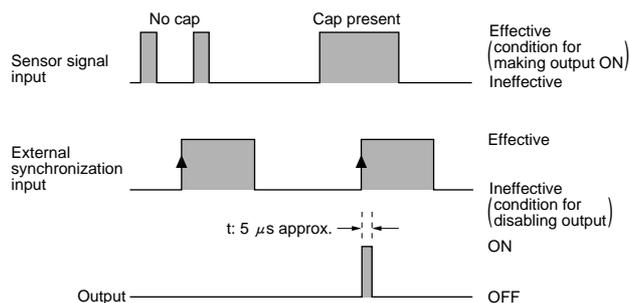
Note: As the output time 't' is only 5 μs approx., extend it by using the OFF-delay timer or the ONE SHOT timer.
