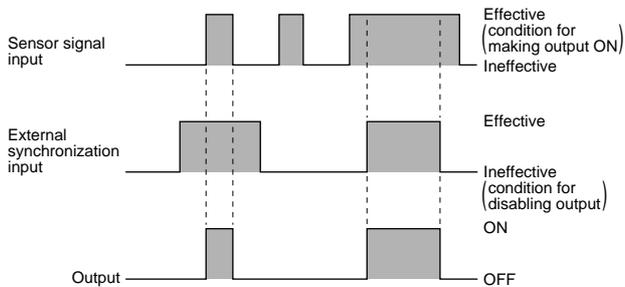
Note: Since NPS-C7 is not incorporated with the selection switch, the output is disabled only when the external synchronization input is Low.
