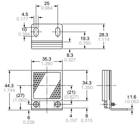
Material: Cold rolled carbon steel (SPCC)
