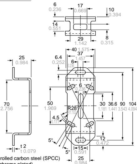
Material: Cold rolled carbon steel (SPCC)
