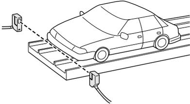
Detecting workpieces on conveyor line
