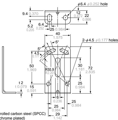
Material: Cold rolled carbon steel (SPCC)
