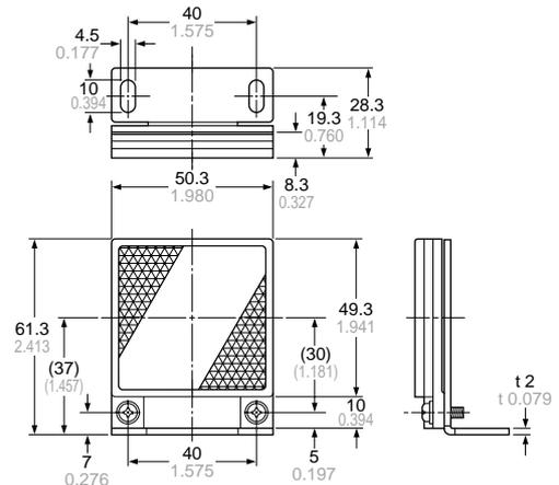
Material: Cold rolled carbon steel (SPCC)
