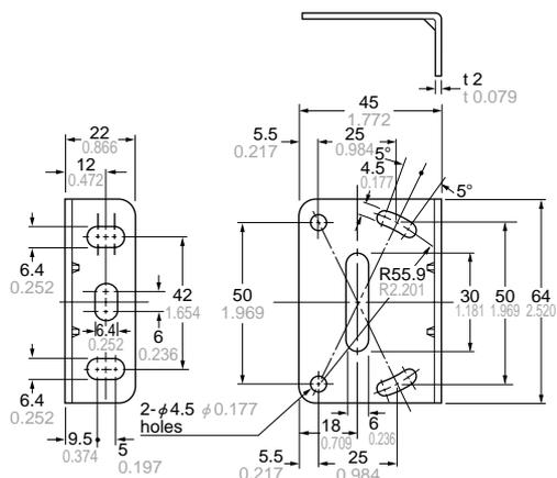
Material: Cold rolled carbon steel (SPCC)
