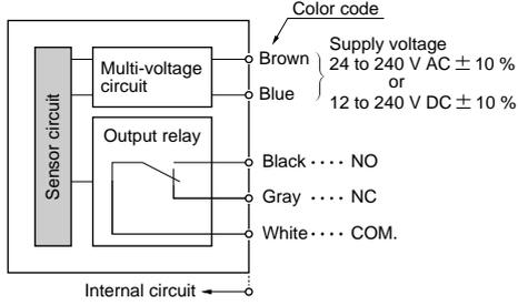
Note: The emitter of the thru-beam type sensor has two wires for power (+ V and 0 V) only.
