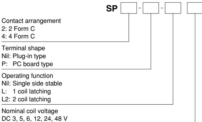
Notes: 1. PC board type and 1 coil latching type are manufactured by lot upon receipt of order.
