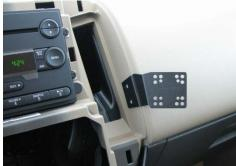
InDash Installed, Mounting Location - Edge
