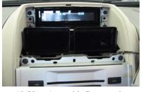
Air Vent Assembly Removed
