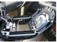
Radio Climate Control, Air Vent, Bezel Removed
