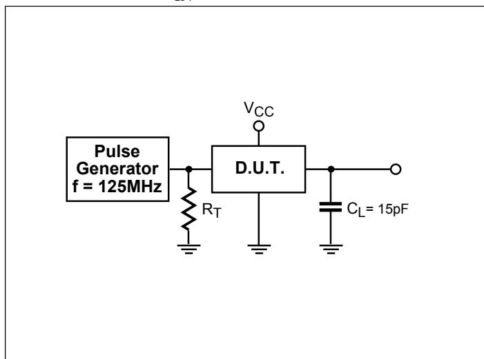
$R_T$  = Termination resistance – should be equal to  $Z_{OUT}$  of the pulse generator
