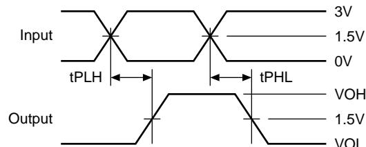
$$t_{SK(p)} = | t_{PHL} - t_{PLH} |$$
