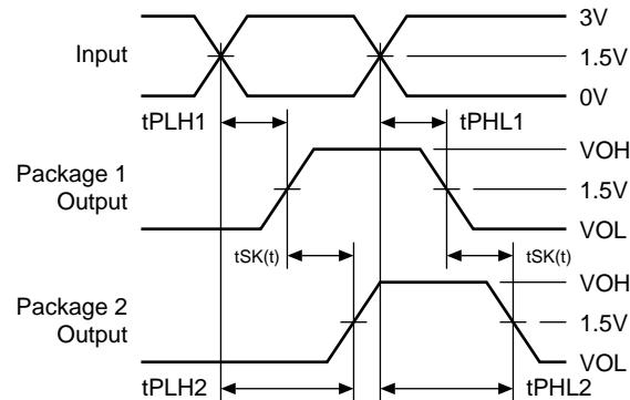
$$t_{SK(t)} = | t_{PLH2} - t_{PLH1} | \text{ or } | t_{PHL2} - t_{PHL1} |$$
