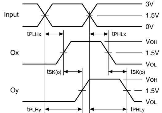
$$t_{SK(o)} = | t_{PLHy} \quad t_{PLHx} | \text{ or } | t_{PHLy} \quad t_{PHLx} |$$
