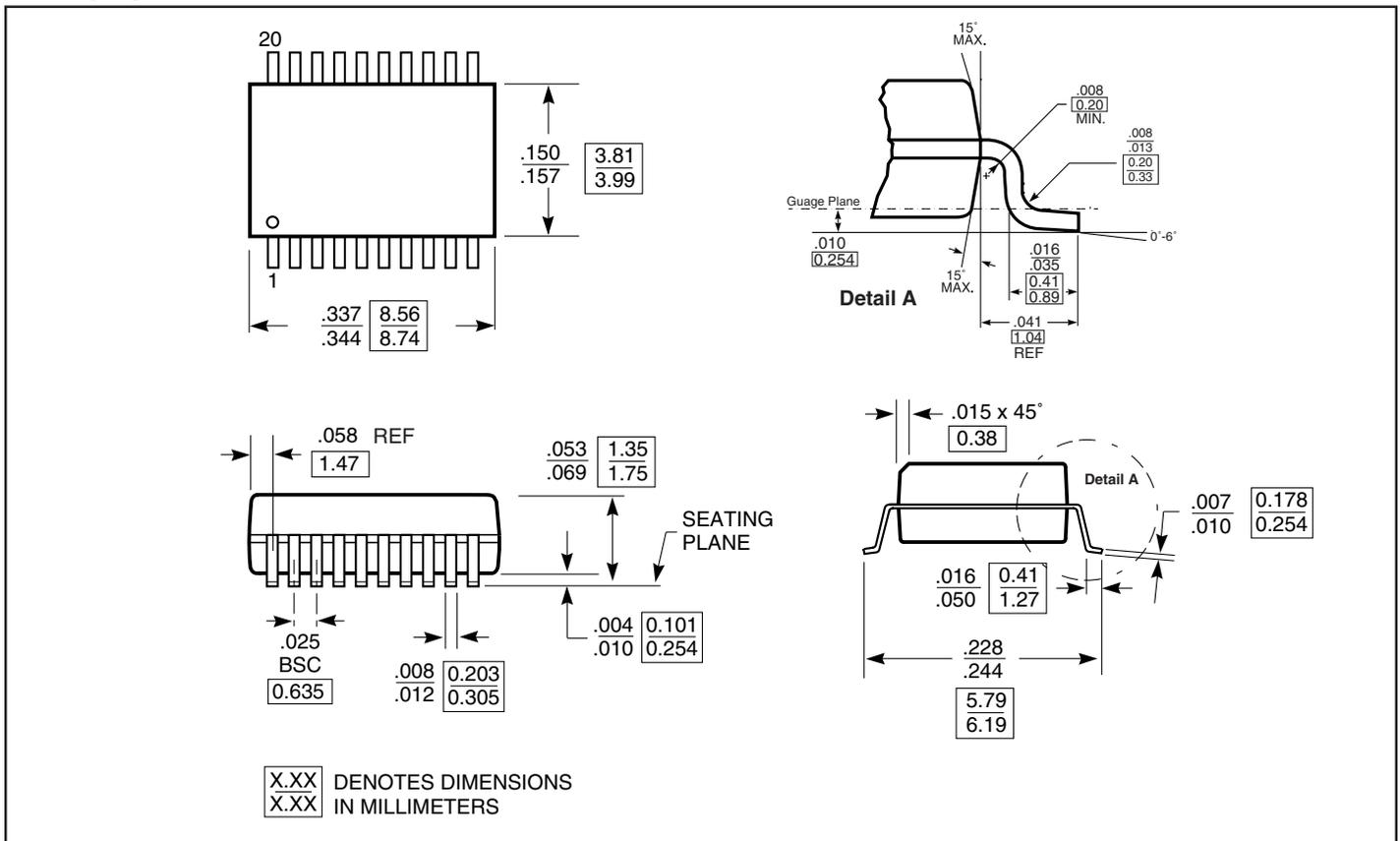
Packaging Mechanical: 20-Pin 300-Mil SOIC (S)
