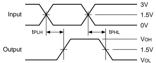
$$t_{SK(p)} = | t_{PHL} \quad t_{PLH} |$$
