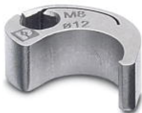
Nut for assembling M8 connectors with longitudinal knurl and a knurl diameter of 12 mm, for 4 mm hexagonal drive
