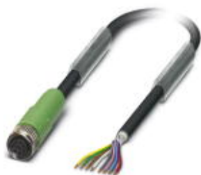
Sensor/actuator cable, 8-position, PUR halogen-free, black-gray RAL 7021, shielded, free cable end, on Socket straight M8, cable length: 1.5 m
