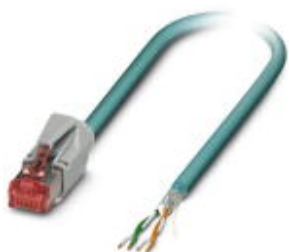
Assembled Ethernet cable, CAT5e, shielded, 2-pair, AWG 26 stranded (7-wire), RAL 5021 (water blue), RJ45 plug/IP20 on free conductor end, line, length 1 m
