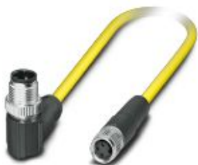
Sensor/actuator cable, 3-position, PVC, yellow, shielded, Plug angled M12 SPEEDCON, coding: A, on Socket straight M8, cable length: 0.5 m
