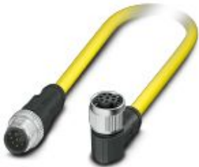
Sensor/actuator cable, 8-position, PVC, yellow, Plug straight M12 SPEEDCON, coding: A, on Socket angled M12 SPEEDCON, coding: A, cable length: 0.5 m
