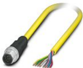
Sensor/actuator cable, 8-position, PVC, yellow, Plug straight M12 SPEEDCON, coding: A, on free cable end, cable length: 5 m
