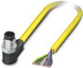
Sensor/actuator cable, 8-position, PVC, yellow, Plug angled M12 SPEEDCON, coding: A, on free cable end, cable length: 5 m
