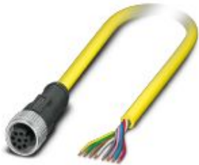
Sensor/actuator cable, 8-position, PVC, yellow, free cable end, on Socket straight M12 SPEEDCON, coding: A, cable length: 5 m
