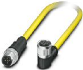
Sensor/actuator cable, 5-position, PVC, yellow, Plug straight M12 SPEEDCON, coding: A, on Socket angled M12 SPEEDCON, coding: A, cable length: 1.5 m
