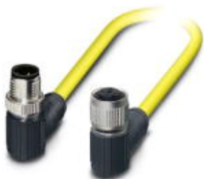
Sensor/actuator cable, 4-position, PVC, yellow, shielded, Plug angled M12 SPEEDCON, coding: A, on Socket angled M12 SPEEDCON, coding: A, cable length: 0.5 m
