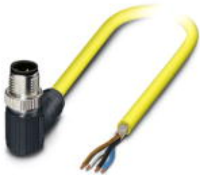
Sensor/actuator cable, 4-position, PVC, yellow, shielded, Plug angled M12 SPEEDCON, coding: A, on free cable end, cable length: 2 m
