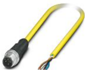
Sensor/actuator cable, 4-position, PVC, yellow, Plug straight M12 SPEEDCON, coding: A, on free cable end, cable length: 5 m
