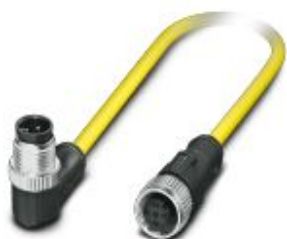
Sensor/actuator cable, 4-position, PVC, yellow, Plug angled M12 SPEEDCON, coding: A, on Socket straight M12 SPEEDCON, coding: A, cable length: 1.5 m
