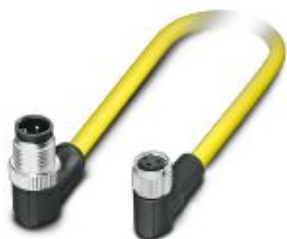
Sensor/actuator cable, 3-position, PVC, yellow, Plug angled M12, coding: A, on Socket angled M8, cable length: 0.5 m
