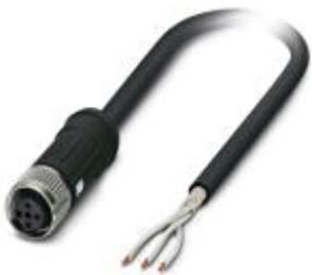
Sensor/actuator cable, 3-position, PE-X halogen-free, black, shielded, free cable end, on Socket straight M12 SPEEDCON, coding: A, cable length: 2 m, For railway applications
