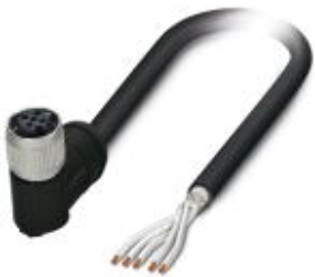
Sensor/actuator cable, 5-position, PE-X halogen-free, black, shielded, free cable end, on Socket angled M12 SPEEDCON, coding: A, cable length: 5 m, For railway applications
