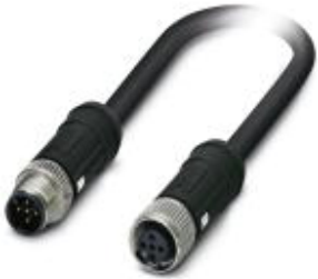
Sensor/actuator cable, 5-position, PE-X halogen-free, black, shielded, Plug straight M12 SPEEDCON, coding: A, on Socket straight M12 SPEEDCON, coding: A, cable length: 5 m, For railway applications
