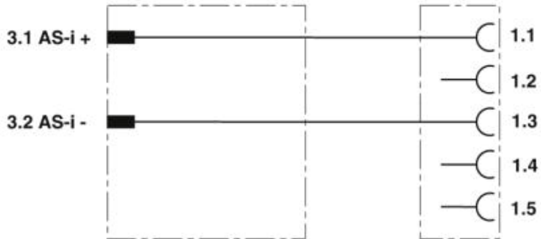
Contact assignment of the AS-Interface distributor
