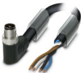
Power cable, 4-position, PUR halogen-free, black-gray RAL 7021, Plug angled M12, coding: T, on free cable end, cable length: 1 m, For direct current up to 12 A/63 V
