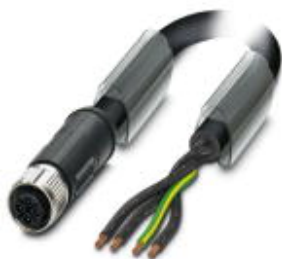
Power cable, 4-position, PUR halogen-free, black-gray RAL 7021, free cable end, on Socket straight M12, coding: S, cable length: 1 m, for AC current up to 12 A/690 V
