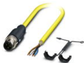
Sensor/actuator cable, 4-position, PVC, yellow, shielded, Plug straight M12 SPEEDCON, coding: A, on free cable end, cable length: 2 m
