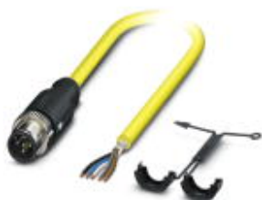
Sensor/actuator cable, 5-position, PVC, yellow, shielded, Plug straight M12 SPEEDCON, coding: A, on free cable end, cable length: 10 m
