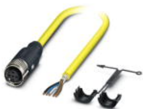
Sensor/actuator cable, 5-position, PVC, yellow, shielded, free cable end, on Socket straight M12 SPEEDCON, coding: A, cable length: 5 m
