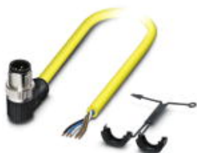
Sensor/actuator cable, 5-position, PVC, yellow, Plug angled M12 SPEEDCON, coding: A, on free cable end, cable length: 2 m
