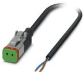
Sensor/actuator cable, 2-position, PUR halogen-free, black-gray RAL 7021, free cable end, on Socket straight DEUTSCH DT06-2S Clip locking, with 1 LED, cable length: 1.5 m, Customer version
