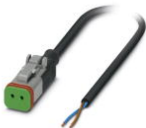
Sensor/actuator cable, 2-position, PUR halogen-free, black-gray RAL 7021, free cable end, on Socket straight DEUTSCH DT06-2S Clip locking, with 1 LED, connected with Diode, cable length: 5 m
