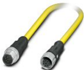
Sensor/actuator cable, 8-position, PVC, yellow, Plug straight M12 SPEEDCON, coding: A, on Socket straight M12 SPEEDCON, coding: A, cable length: 5 m
