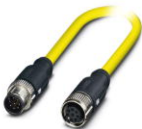
Sensor/actuator cable, 8-position, PVC, yellow, shielded, Plug straight M12 SPEEDCON, coding: A, on Socket straight M12 SPEEDCON, coding: A, cable length: 20 m
