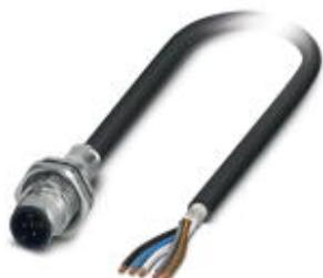
Flush-type plug, shielded, 5-pos., M12, A-coded, rear/screw mounting with M16 thread, with 2 m cable, 5 x 0.34 mm<sup>2</sup>
