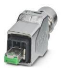
Push-pull connector (version 14), die-cast zinc, with RJ45 connector insert, 8-pos., with IDC fast connection technology, for 1 and 7-wire cores, 23 ... 22 AWG, for cable diameter of 5.5 mm ... 10 mm
