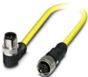
Sensor/actuator cable, 5-position, PVC, yellow, Plug angled M12 SPEEDCON, coding: A, on Socket straight M12 SPEEDCON, coding: A, cable length: 1.5 m
