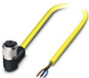
Sensor/actuator cable, 3-position, PVC, yellow, free cable end, on Socket angled M12 SPEEDCON, coding: A, cable length: 15 m
