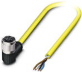
Sensor/actuator cable, 4-position, PVC, yellow, free cable end, on Socket angled M12 SPEEDCON, coding: A, cable length: 15 m
