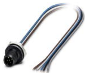
Sensor/Actuator flush-type connector, male, 5-pos., M12, A-coded, front/screw mounting with M16 thread, with 0.5 m TPE litz wire, 5 x 0.25 mm², plastic version
